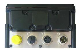
» If the LEDs above the connectors light up, you can be sure that the device has power supply
