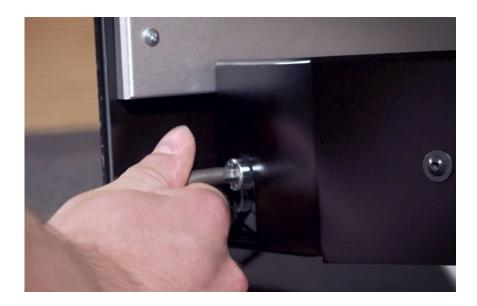
> Carefully rotate the panel by 90° to the front. Secure the glass. No force should ever be applied:
