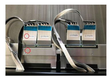
o Use the provided grey sticker to fix and shield the cable to the socket:
