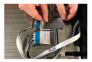
Put the PCB covers back while guiding the flexible flat cables back through the holes with caution:
