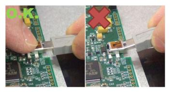
Note: Avoid breaking the sockets by wrong handling
