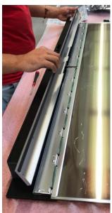
> Remove the screws with the green mark to rise the inside PCB covers:
