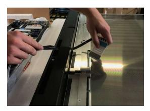
Clean the contacts of the flexible flat cables with isopropanol and insert them into the sockets with caution. Make sure the connectors are inserted correctly:
